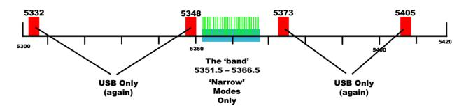
This diagram adds the option of a 'wide' digital segment as a suggestion. It also shows what spectrum would be available to a radio that currently has the capability to operate as USB on the existing 5 channels, but would have to be modified (if possible) to take advantage of the new 15 kHz wide band.
